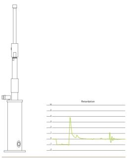
**Fly ball governor** A fly ball governor detects abnormal speed and activates an emergency stop when necessary. Speed can be precisely measured even during ultra high speed operation, resulting in a level of safety that befits the elevator's class.
