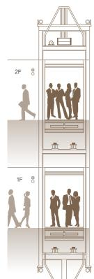
**Higher transport efficiency** Two elevators connected vertically are simultaneously run to offer 1.8 times greater transport capability. Fewer hoistways mean lower construction costs and more available floor space.
